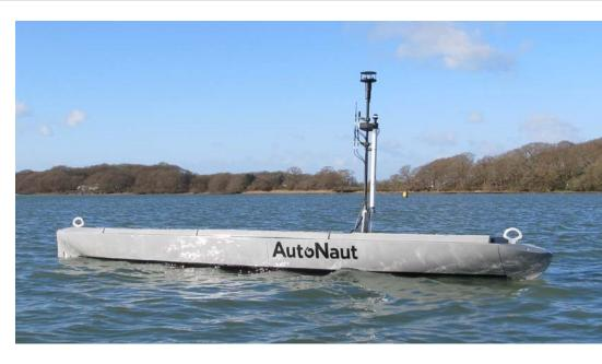
In June 2017 AutoNaut deployed their wave-powered unmanned surface vessel (USV) "Islay" around the Swedish Island of Gotland. Islay is a 5-metre AutoNaut and this vessel enabled the Swedish University of Agriculture and Sciences, Department of Aquatic Resources, to fit the sensors they required to monitor fish stocks in the North Atlantic and Baltic Seas.
